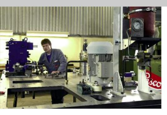
LASCO employees are installing the hydraulic drive of a VPE.
