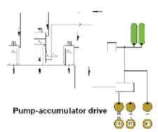
The pump-accumulator drive stores part of the energy in the accumulator. This solution is preferred when high pressing speeds are necessary, but production output is not high, allowing time for recharging the accumulator, between press strokes, and reducing the size of the motors installed.
