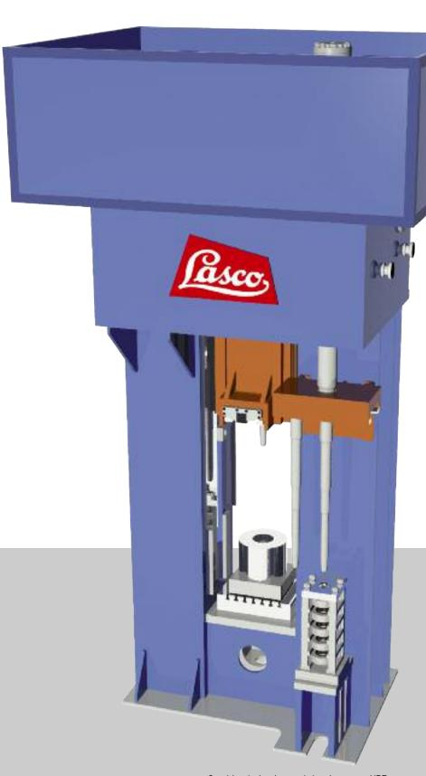
Combined piercing and drawing press VPZ for the production of axially symmetrical parts (schematic).
