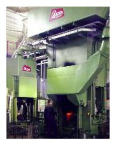
Pistons are forged on a VPE 160 and a VP 800.
