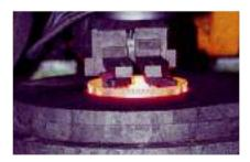
Hot calibration of powder-forged synchronous rings.
